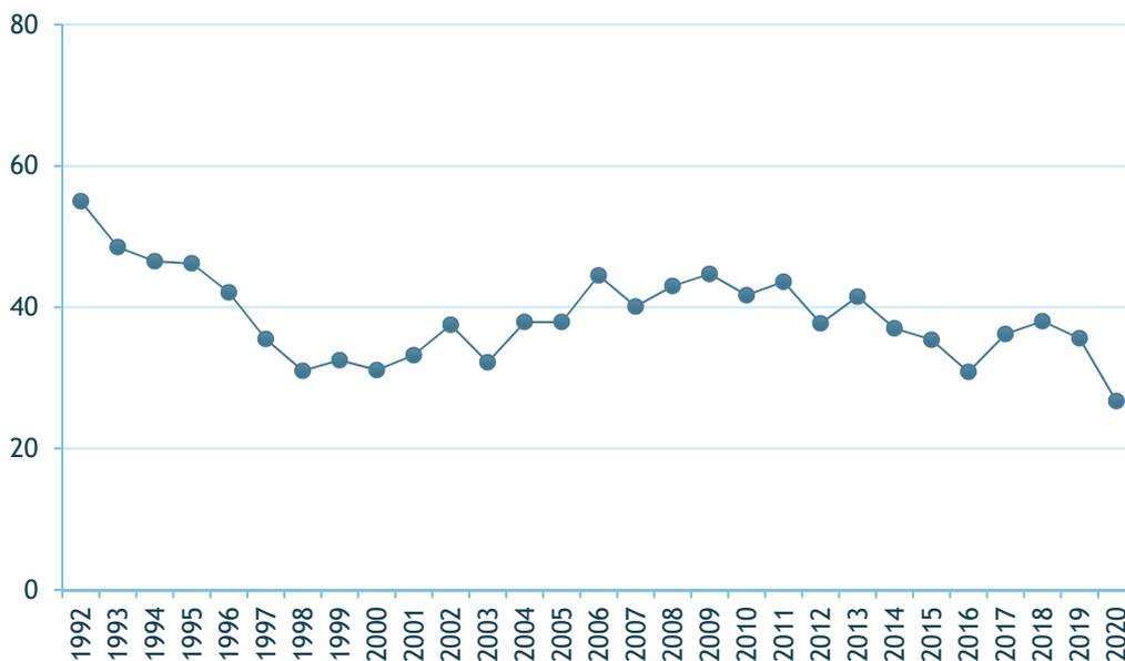
Figure 35: Fluoride emissions (tonnes per year) from Alcoa Lista from 1992 to 2020. Source: AMS.
