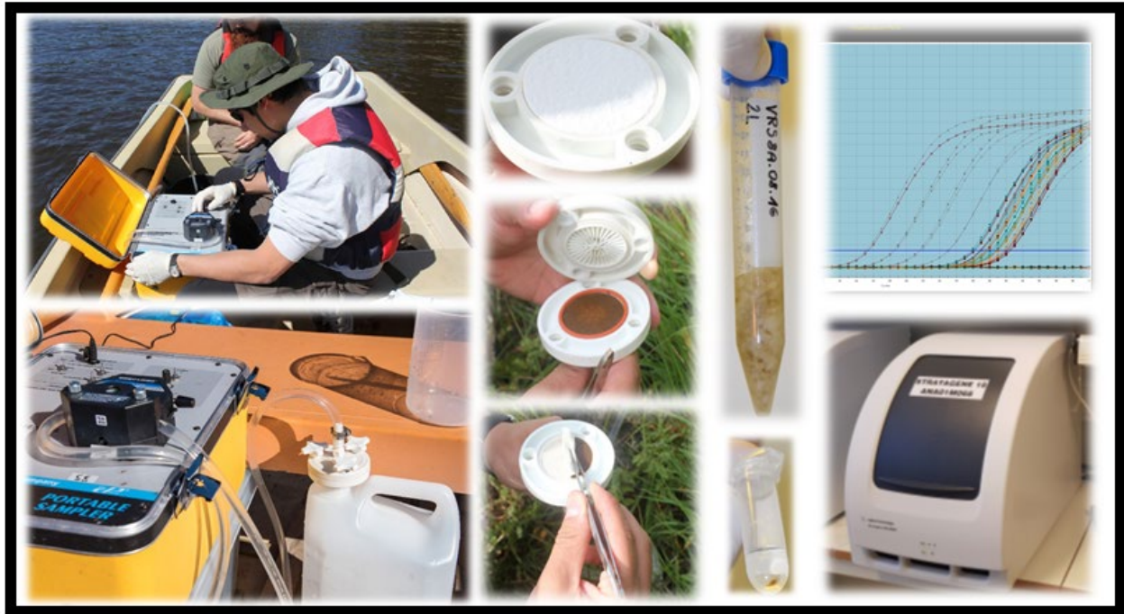
Figure 5. Water samples of ~5 L each were filtered on-site through glass fibre filters using a portable peristaltic pump (Masterflex E/S portable sampler). Each filter was carefully transferred to a 15ml tube with buffer and stored there, until further processing in the laboratory. DNA was isolated with a large volume extraction procedure and presence/absence of eDNA from all target organisms was analysed using qPCR. Figure modified from Vrålstad et al. 2016 [7].
